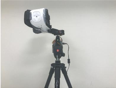
Fig. 9. Our VR testbed consists of a GearVR, an S7, a Pan/Tilt mount, a 3D-printed holder for the mount, a Raspberry Pi to accurately control the mount's motion, and a tripod for stabilizing the test instruments.
