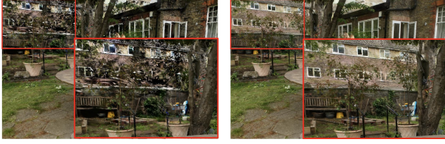
(a) View rendered with the ViVo approach. PSNR = 17.48 dB (b) View rendered with our SGSS approach. PSNR = 22.21 dB Figure 9: Side-by-side comparison: rendering result of garden at the 22th second under 200 Mbit/s bandwidth.
