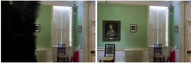
(a) View rendered with the DWO approach. PSNR = 10.71 dB (b) View rendered with our SGSS approach. PSNR = 30.66 dB
