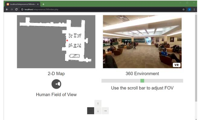
Fig. 3: *Telepresence Interface* showing the 2D map, the frame of the remote environment, a 2D icon to show human head orientation, a scrollbar to adjust field of view, and a set of icons to indicate the current teleoperation commands given by the human operator.
