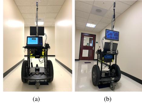
Fig. 1: Segway-based mobile robot platform (RMP-110) with a 360-degree camera (Ricoh Theta V), mounted on top of the robot, and laser rangefinder (SICK TiM571 2D) that has been used for prototyping and evaluation purposes in this research.
